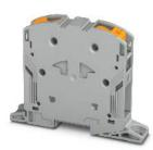
High-current terminal block, nom. voltage: 1000 V, nominal current: 232 A, connection method: Power-Turn connection, 1 level, cross section: 25 mm<sup>2</sup> - 95 mm<sup>2</sup>, mounting type: direct screw connection, color: gray
