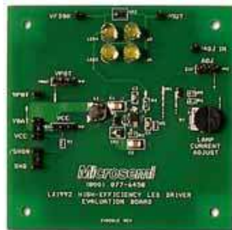
Figure 5: LX1992 Engineering Evaluation Board
