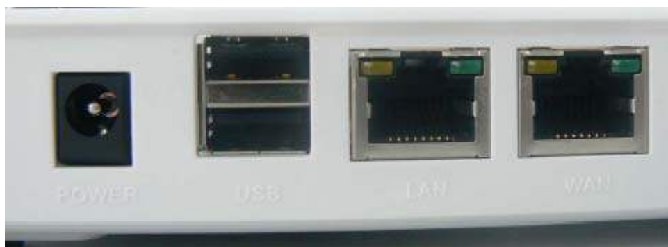
Figure 3. Ethernet and USB Ports on MPC8308-NSG
