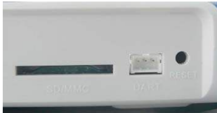
Figure 4. UART Port and SD/MMC Slot on MPC8308-NSG
