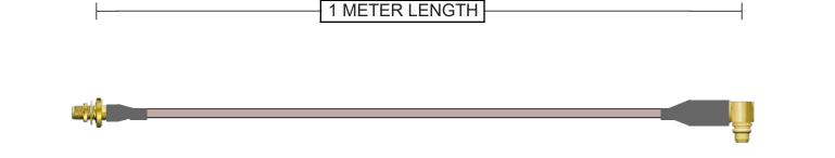
Connector A 132286 SMA Jack Straight Bulkhead - Rear Mount Brass Gold + Heatshrink 50 Ohm RG-178 Continuity/Hi-Pot Connector B 262102 MMCX Plug Right Angle Brass Gold + Heatshrink
