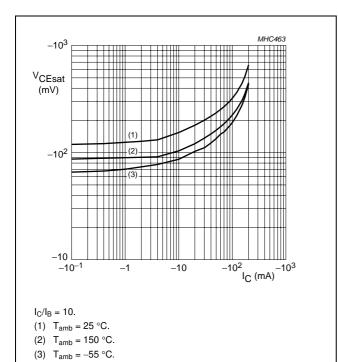
Fig.6 Collector-emitter saturation voltage as a function of collector current.
