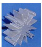
Wakefield's new 882 series heat sinks can be used with LEDs in the star package from Lumileds, Osram, and others. The radial design and fin area is ideally suited for natural convection applications such as ceiling lighting. A fan can also be used for increased performance in a forced convection application. Three sets of mounting holes allow maximum flexibility.
