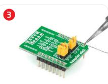
Turn the board upward again. Make sure to align the headers so that they are perpendicular to the board, then solder the pins carefully.
