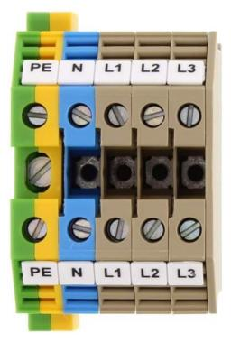
Five-wire mains-connection block, Screw connection, Mounting type:Mounting rail TS 35/7.5 and TS 32, Rated cross-section: 4 mm<sup>2</sup>, Colour: Multi-coloured
