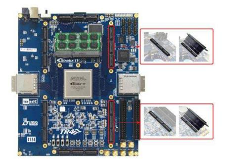
Connection between HMF2 Adapter Card and DE4 board
