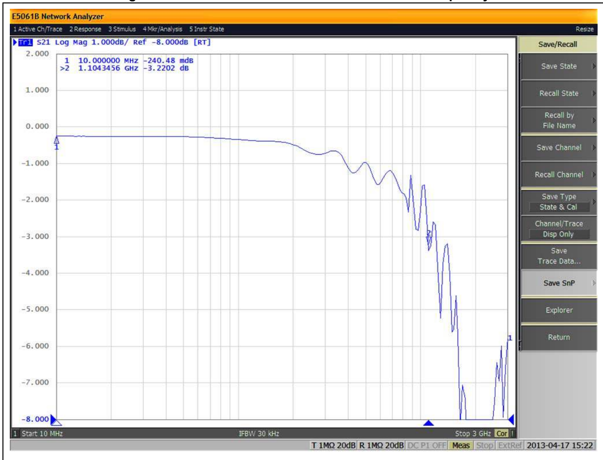
Figure 22. Data switch transfer characteristics vs. frequency
