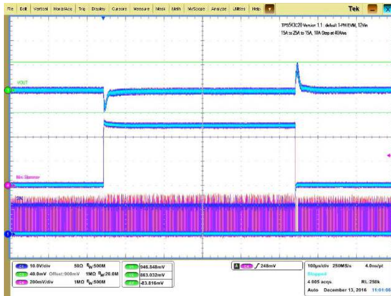
Figure 7. Transient Response of 0.9-V Output at 12-V IN , Transient is 15 A to 25 A to 15 A, the Step is 10 A at 40 A/μs
