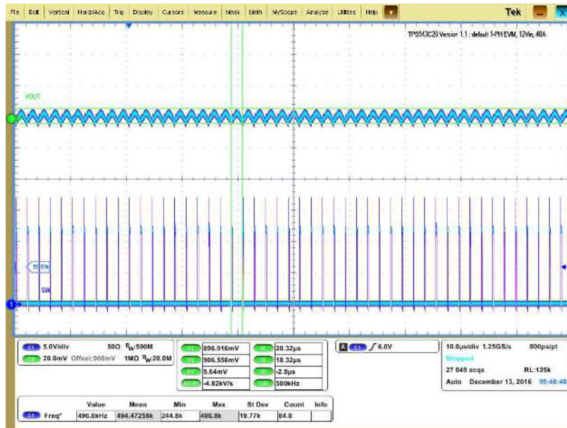
Figure 8. Output Ripple and SW Node of 0.9-V Output at 12-V IN , 40-A Output
