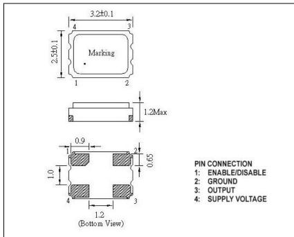
NOTE: A capacitor of 0.01 µF between Vcc and Ground is recommended
