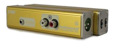
The 370DI is a durable, pocket size, Direct Box which is a cross between Switchcraft's SC700CT DI Box and 318 Inline Audio Adapter. The 370DI sums and converts the unbalanced stereo outputs of cell phones, tablets, laptops and consumer gear to a balanced mono line level for connecting to audio consoles and house sound systems.
