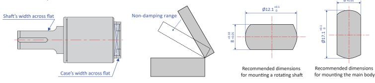
■ The damper's working angle is 115°, as shown below. Rotating the damper beyond this angle will cause damage to the damper. Please ensure that an external stopper is in place. The working angle is based on the width across flat for fixing, located towards the rear end of the main body. The position where the rotation is complete is at 90° with respect to the width across flat.
