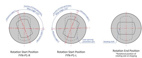
The direction in which torque is generated varies according to the model.
