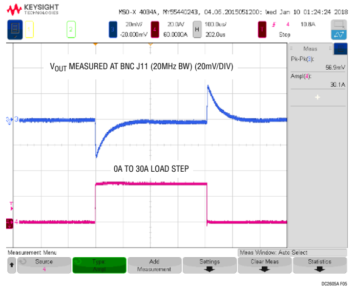
Figure 5. Transient Response at V_{IN} = 12V , V_{OUT} = 1V , f_{SW} = 425kHz
