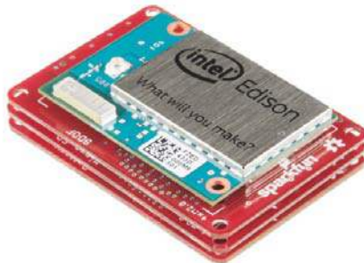
9 DOF Block Installed
