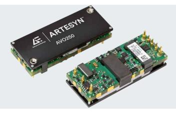
Advanced Energy's Artesyn AVO250 series eighth-brick isolated DC-DC converter provides a single regulated low noise 28 Vdc output. The converter has a wide 2:1 input range of 36 to 75 Vdc and is designed primarily for use with standard 48 V telecommunications equipment supplies. Rated at 250 watts, it can deliver up to 9 amps and accommodates an ambient operating temperature range of -40 to 85°C.
