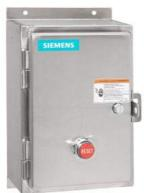
Non-reversing motor starter, Size 3 1/2, Three phase full voltage, Solid-state overload relay, OLR amp range 50-200A, Non-combination type, Encl. type 4X 304 S. Steel, Water/dust tight noncorrosive, Standard width enclosure
