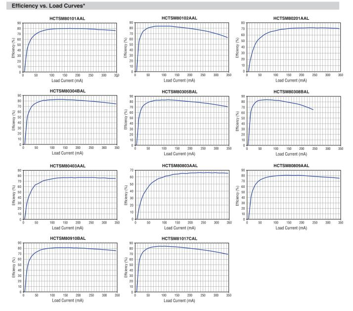
\*Measured with circuit in Typical Application, 5 VDC input, 0-350 mA DC load, Ta = 20 °C
