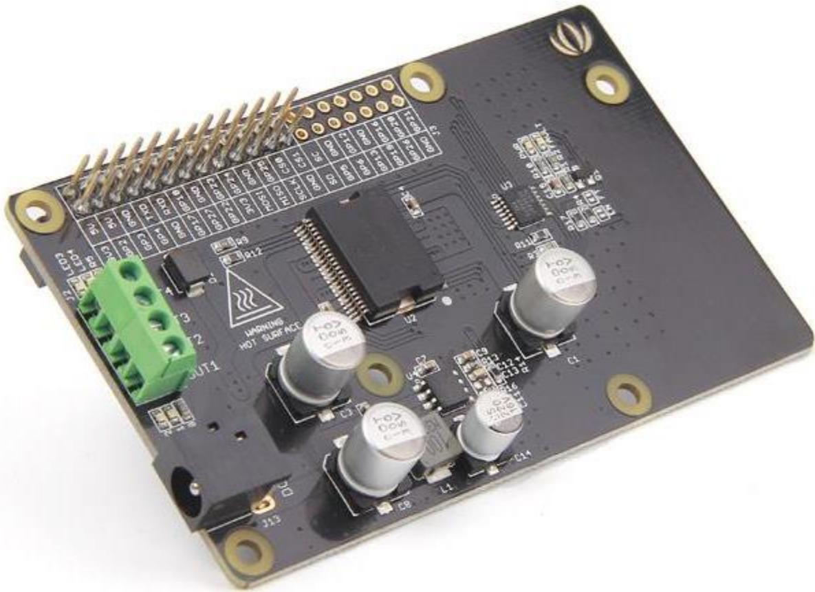
Raspberry Pi Motor Driver Board v1.0 is based on the Freescale MC33932 dual H-Bridge Power IC, which can control inductive loads with currents up to 5.0A peak per single bridge. It lets you drive two DC motors with your Raspberry Pi B/B+/A+ and Pi 2 Model B, controlling the speed and direction of each one independently.
