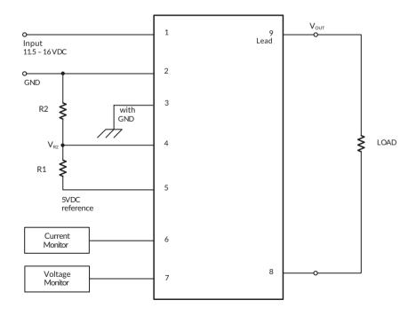
Operate with 5VDC Reference Voltage Variable output
