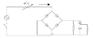
Ct2 Test capacitance [µF] Imax2 Max current across the NTC under test [A] Number of cycles: 1000
