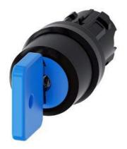
Key-operated switch O.M.R, 22 mm, round, plastic, lock number 73038, blue, with 2 keys, 3 switch positions I-O-II, latching, actuating angle 2x45°, 10:30h/12h/13:30h, key removal O, with laser labeling, inscription or symbol Customer-specific selection with SIRIUS ACT configurator (CIN)
