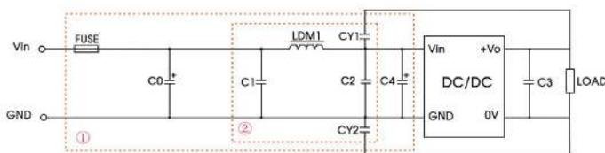
Notes: Part ① is used for EMC test and part ② for EMI filtering; selected based on needs.
