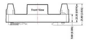
Note: Unit: mm[inch] Wire range: 24-12 AWG Tightening torque: Max 0.4 N·m Mounting rail: TS35 General tolerances: ±1.00[±0.039]
