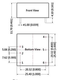
Note: Unit: mm[inch] Pin diameter tolerances: ±0.10[±0.004] General tolerances: ±0.50[±0.020] THIRD ANGLE PROJECTION 💮 🖯
