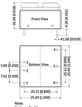
Unit: mm[inch] Pin diameter tolerances: ±0.10[±0.004] General tolerances: ±0.50[±0.020]
