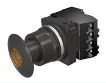
30mm BlackMax, Epoxy Coated Corrosion Resistant Complete Metal Unit Illuminated Push-Pull Operator Transformer type, 240V AC LED Lamp Mushroom Head Cap Small 1 3/4" (44.5 mm) Metal, Black with Amber Lens 2 Position Maintained, Pull-to-Release with 1 N.O. - 1 N.C. Heavy Duty Contacts, A600/P600 UL Listed, CSA Certified NEMA 1,3,3R,4,4X,12,13 & Automotive Standards
