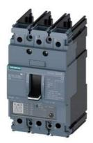
circuit breaker 3VA5 UL frame 125 3-pole, starter protection TM120M, FM, In=15A without overload protection short-circuit protection Ii=5...12 x In without connection
