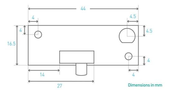
The 2 mounting holes are 3.3mm diameter.
