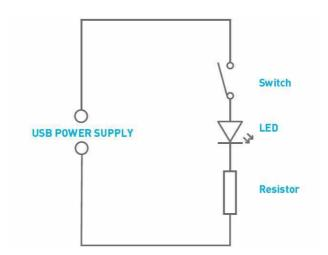
The circuit diagram for the USB lamp is shown above. It is a very simple circuit. The 5V that powers the circuit is supplied from the USB connector.
