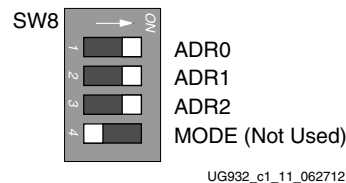
Figure 1-11: Configuration Address DIP Switch (SW8)
