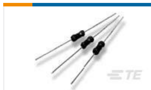
TE Part #4-1625890-5 2W SM M/OX 5% 39K
