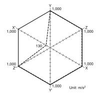
Test conditions: Shock is applied in  $\pm X$ ,  $\pm Y$ , and  $\pm Z$  directions three times each with without energizing the Relays to check the number of malfunctions.
