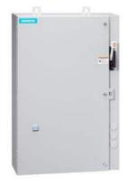
Non-reversing motor starter, Size 4, Three phase full voltage, Solid-state overload relay, OLR amp range 50-200A, 24VAC 50-60Hz coil, Combination type, 200A fusible disconnect, 200A/600V fuse clip, Enclosure NEMA type 4/12, Water/dust tight for outdoors, Standard width enclosure
