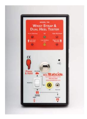
Easy to use: Position selector switch according to desired test: wrist, feet, or both simultaneously. Step on footplate then press and hold the button. The green "OK" LED will illuminate for a pass and one of the red LEDs will illuminate for a failure. A buzzer will also sound for failed tests. Red lights will signify whether an employee tested too high or too low, or whether there was a wrist strap failure or a heel grounder failure. Details of testing are found in the ACL 780 manual.
