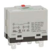
Harmony, Power relay, with plugin socket, 25 A, with LED and flag indicator, with lockable test button, 120 V AC, 2 NO, flat (faston) terminals
