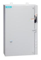
Non-reversing motor starter, Size 1, Three phase full voltage, Solid-state overload relay, OLR amp range 0.25-1A, Combination type, 30A fusible disconnect, 30A/600V fuse clip, Enclosure NEMA type 4/12, Water/dust tight for outdoors, Extra-wide enclosure
