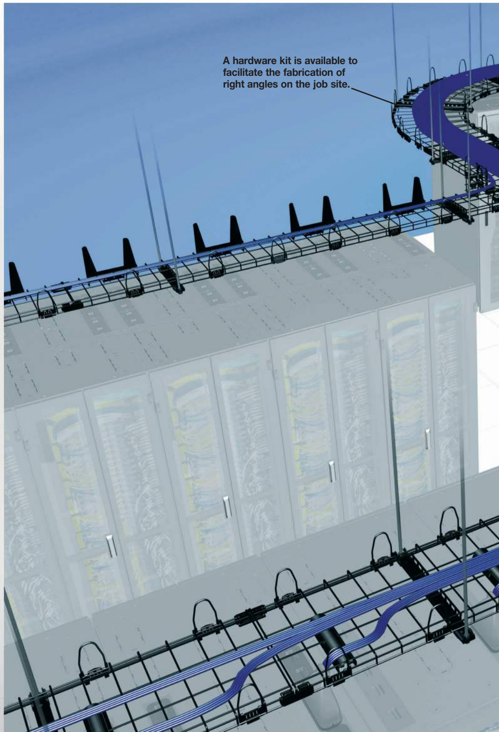
Route redundant ("A" and "B") cabling into adjacent cabinets with a single waterfall.
