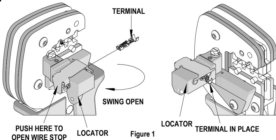
**CAUTION:** Install only Molex terminals listed above with this tool. Do not crimp hardened objects as damage can occur to the tool or die.
