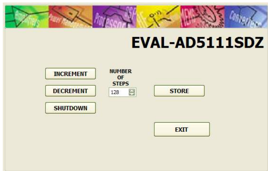
Figure 5. EVAL-AD5111SDZ Evaluation Board Software Main Window
