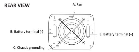
A: Fan: Do not obstruct, allow at least 12 inch for air flow.
