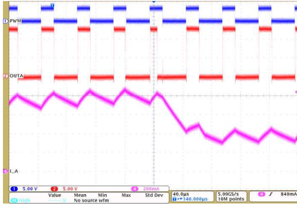
Figure 9-15. Driver PWM Operation with Current Limit
