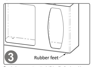
For placing on counter, attach (4x) self-adhesive rubber feet at each of the bottom corners (included).
