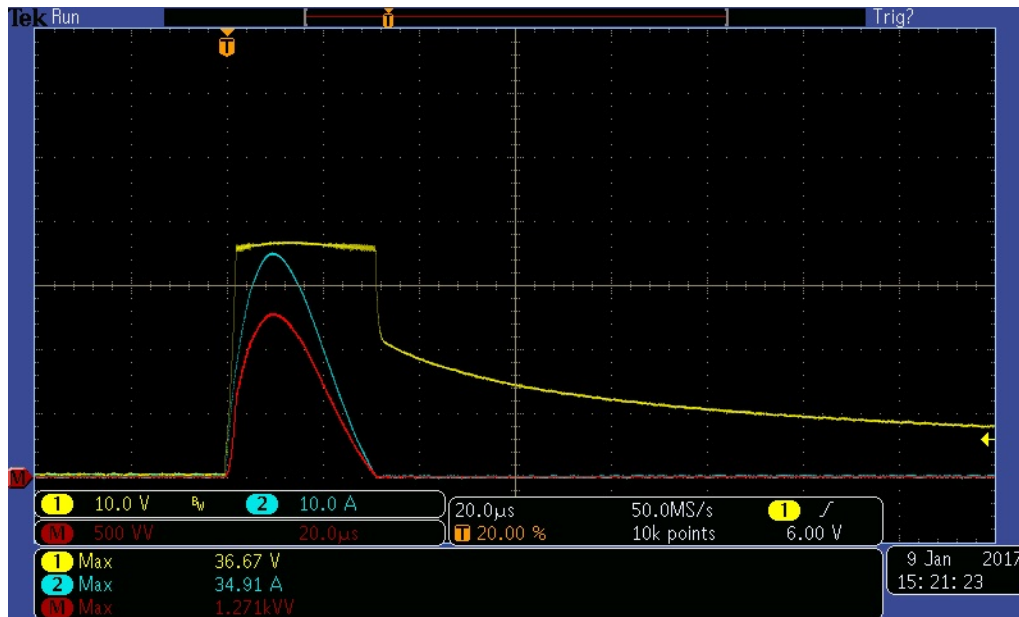
Figure 6. TVS3300YZF Surge Test Waveform
