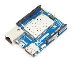
The Yún rev. 2 with the power of a Linux based system that enables advanced network connections and applications.
