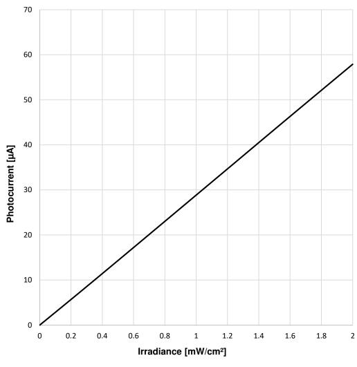
Testcondition: Ee=0,5mW/cm<sup>2</sup>, VR=5V
