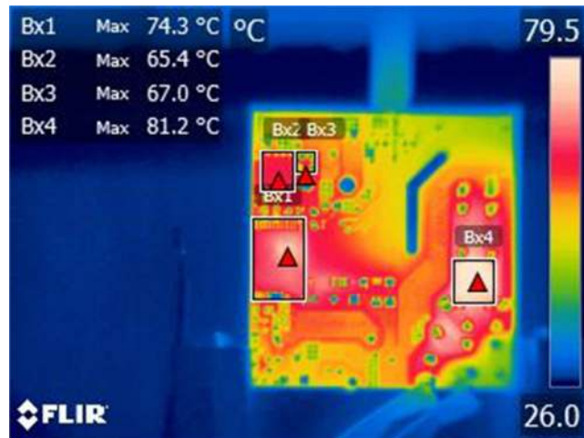
Figure 42 – Bottom Thermal Image, T_{AMB} = 26.0 °C. Bx1: InnoSwitch3-PD, U_1 = 74.3 °C. Bx2: SR FET, Q_2 = 65.4 °C. Bx3: SR FET Snubber, R_{10} = 67.0 °C. Bx4: Bridge Rectifier, BR_1 = 81.2 °C.
