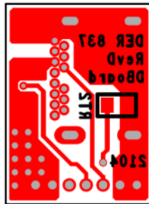
Figure 9 – DER-837 RevD USB Type-C Connector PCB Layout, Bottom.
