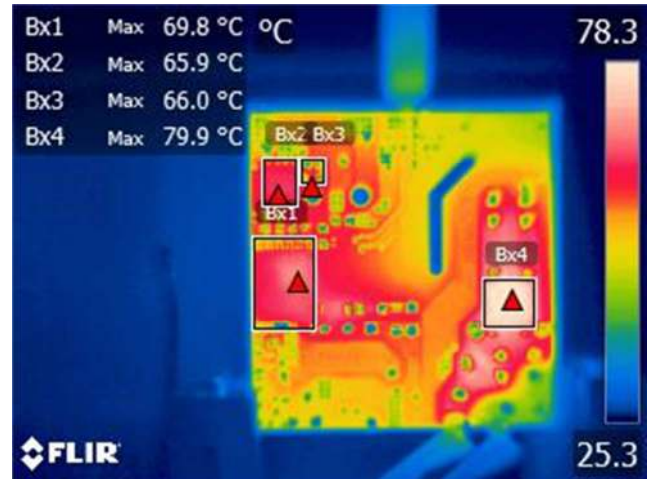
Figure 38 – Bottom Thermal Image, T_{AMB} = 25.2 °C. Bx1: InnoSwitch3-PD, U_1 = 69.8 °C. Bx2: SR FET, Q_2 = 65.9 °C. Bx3: SR FET Snubber, R_{10} = 66.0 °C. Bx4: Bridge Rectifier, BR_1 = 79.9 °C.
