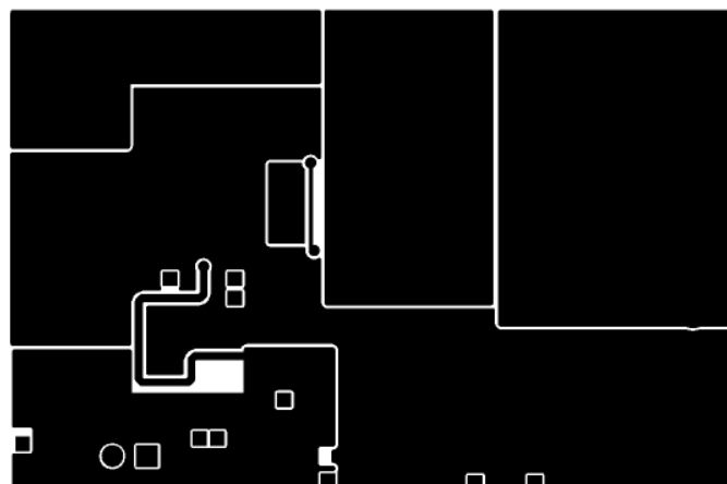
Figure 41. TPS40200EVM-001 Bottom Copper (X-Ray View from Top)
