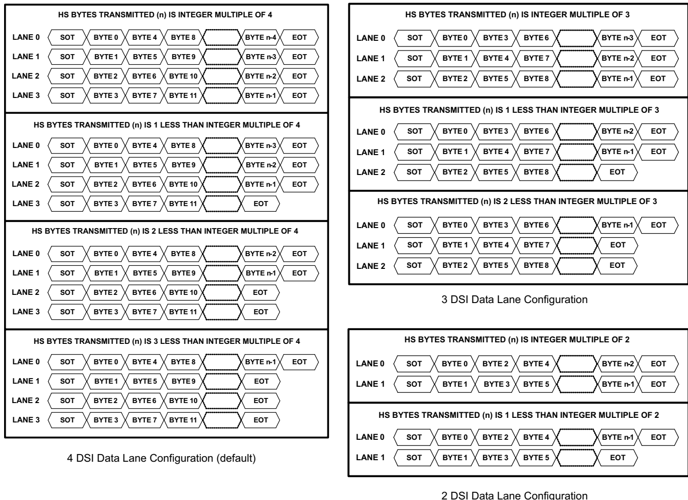
Figure 13. SN65DSI83-Q1 DSI Lane Merging Illustration
