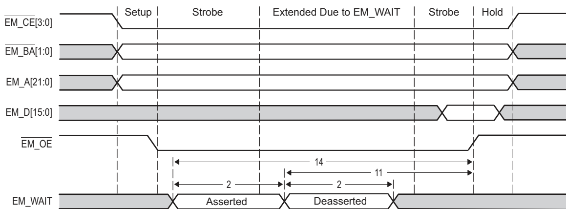
Figure 5-22. EMIF16 EM_WAIT Read Timing Diagram
