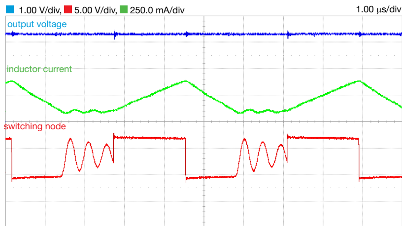
Figure 7. V_{in}=6V , I_{out}=0.1A , f_s=250kHz
