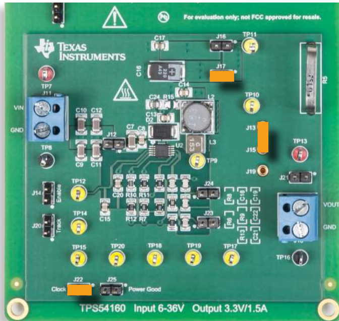
Figure 6. TPS54160 buck board: jumpers set-up for Test#2
