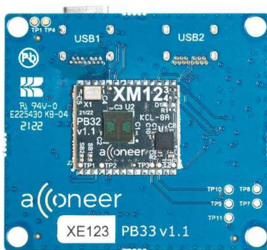
Picture 1. The XE123 top side where XM123 is mounted.
