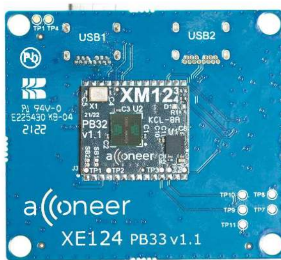
Picture 2. The XE124 top side where XM124 is mounted.
