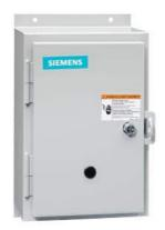
Non-reversing NEMA contactor, Size 1, Three phase full voltage, Contactor amp rating 27A, 3 wire (NO aux included), 220-240/440-480VAC 60Hz coil, Non-combination type, Enclosure NEMA type 12, Dust/drip proof for indoors, Extra-wide enclosure
